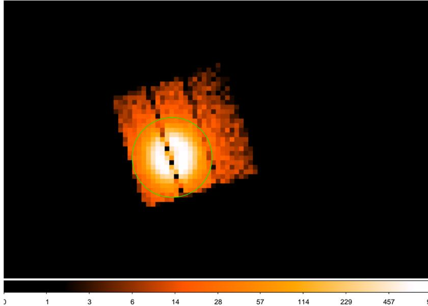
Figure 5: MOS-1 sky coordinate image of 1E0102-72.2. The green circle indicates the region used to extract the MOS-1 spectrum which contains a bad column.
