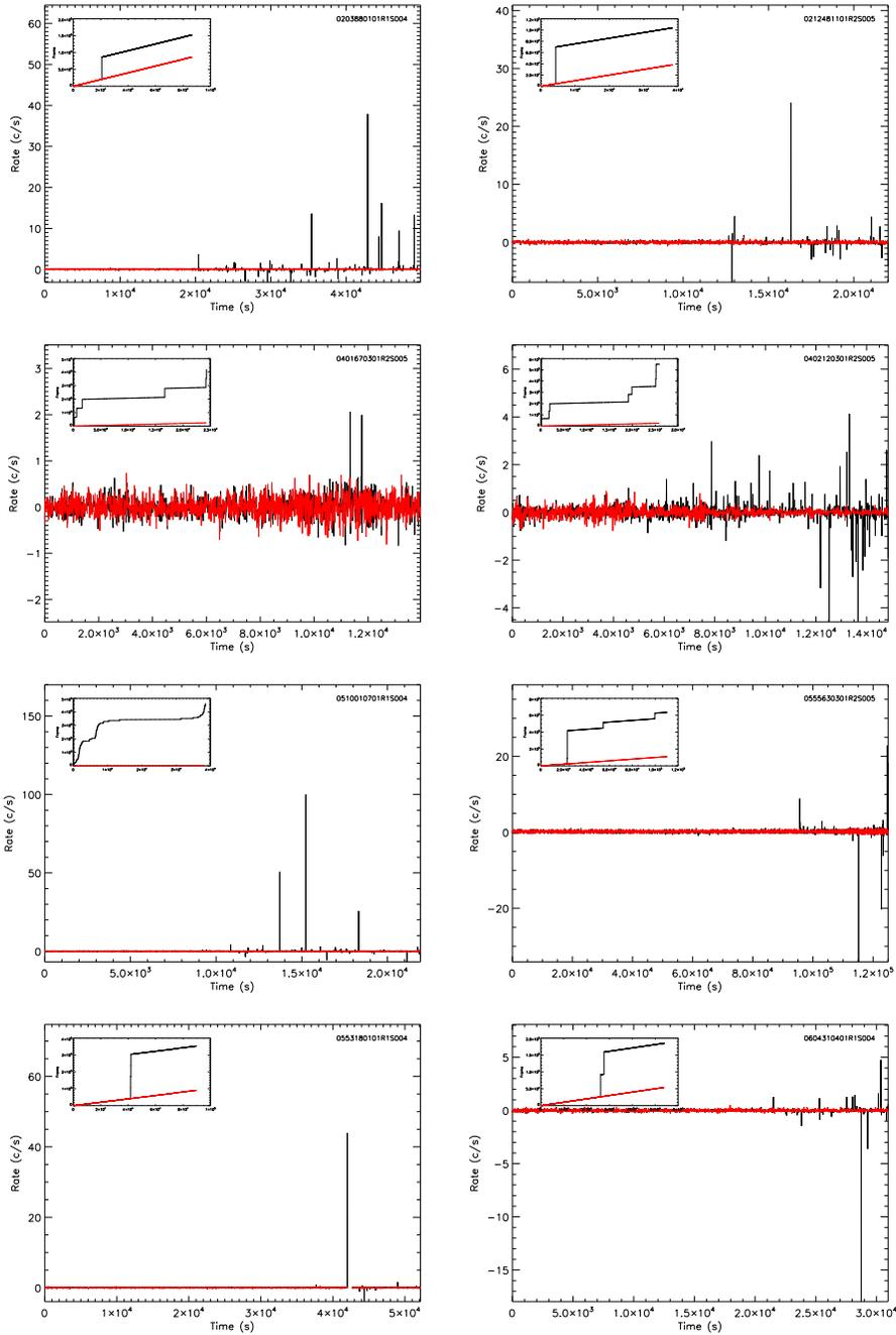
Figure 4: Examples of light curves corrected for frame jumps. Shown in black are data processed with SASv16, in red with SASv17 after correction with `rgsframejumpfix`. The inset shows the frame counter.
