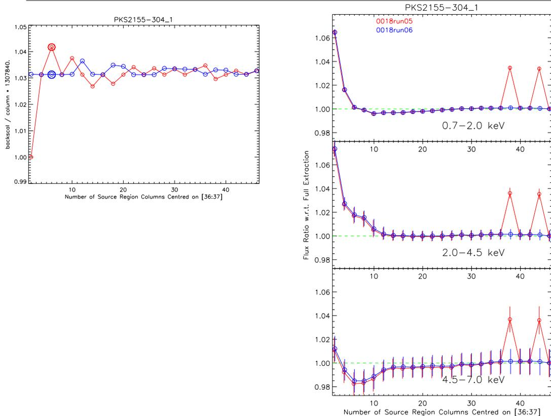
Figure 3: Left: Area of the source extraction region for a Timing mode observation as calculated by `backscal` against the number of columns used in the extraction (SAS 16.0.1: red curve; SAS 17: blue curve). Right: ratio of returned flux for source extractions of increasing number of columns, compared with that obtained from the full extraction area, for energy ranges of 0.7–2, 2–4.5 and 4.5–7 keV.
