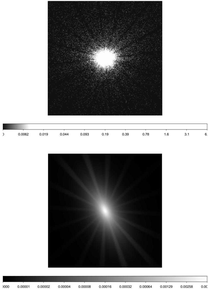
Figure 6: Upper: example 3 of psfgen user guide - MEDIUM mode MOS1 PSF at 3 arcminutes off-axis and energy of 3keV. Lower: example 5-1 from the psfgen user guide - ELLBETA mode PSF of energy 3 keV at  $\sim 9$  arcminutes off axis.
