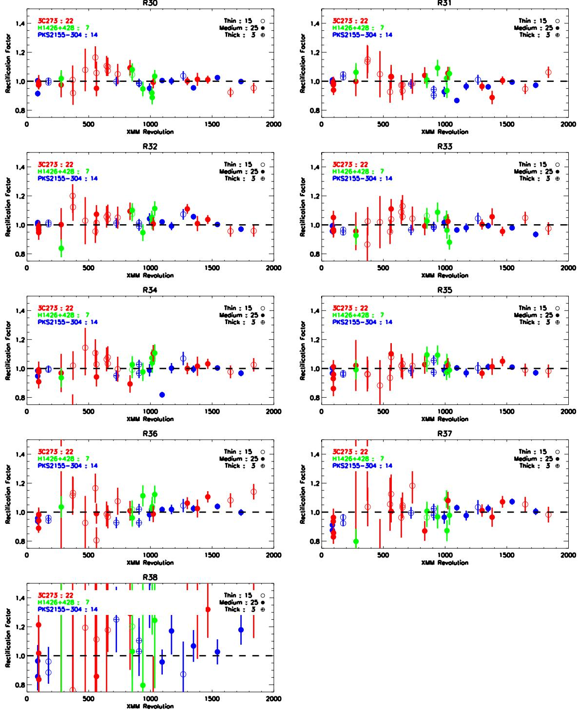
Figure 6: Time evolution of the individual RGS 1 rectification factors.
