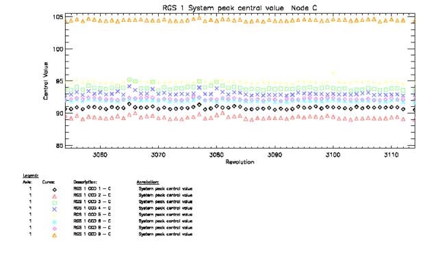
Figure 2: Fig. 1 - Main offset values per  $\operatorname{CCD}$  -  $\operatorname{C}$  side in the last 60 revolutions
