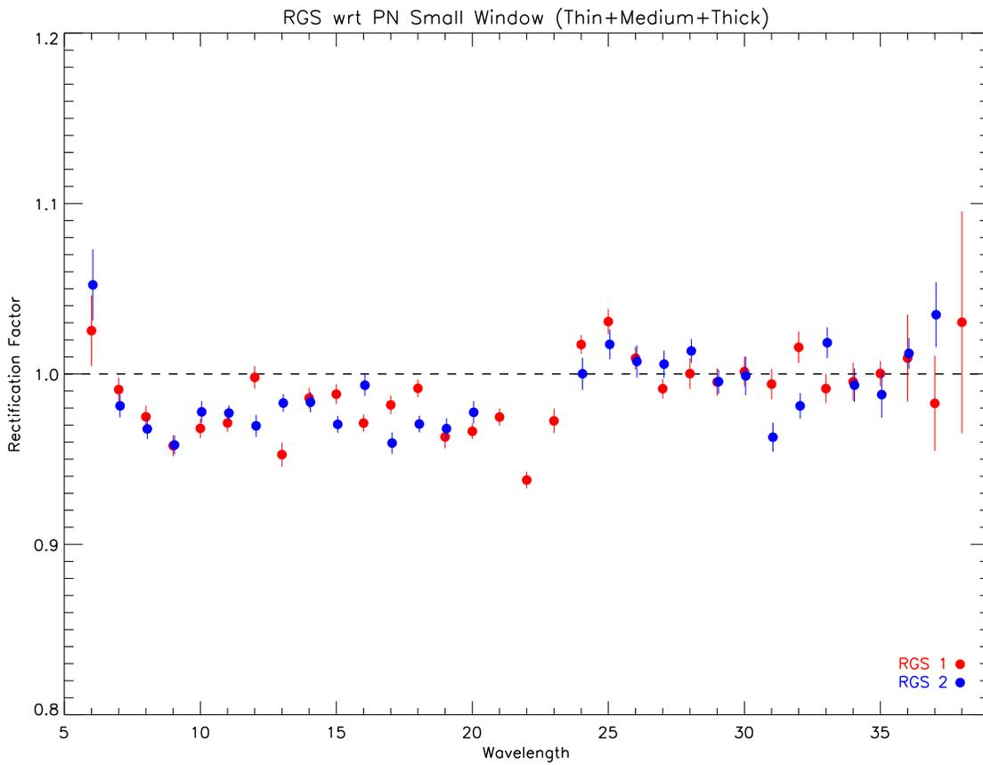
Figure 1: Average RGS1-pn and RGS2-pn rectification factors in 1Å intervals for XCal models of a standard sample of AGN including 3C273, PKS2155-304, H1426+428 and other sources. This is Figure 12 from [3] and suggests that a smooth approximation could be provided by a step function at the oxygen edge, separately for RGS1 and RGS2.
