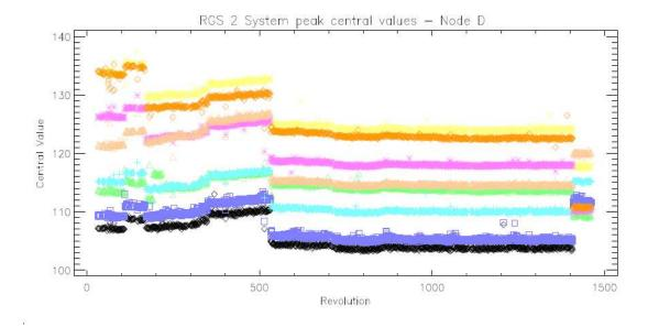
Figure 1: Evolution of RGS2 node D system peak value throughout the whole mission. The different colours and symbols represent the 8 different CCDs. Large stability is observed after revolution 535 when the operating temperature was lowered
