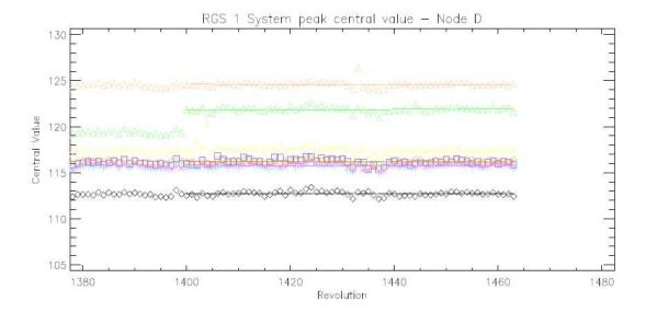
Figure 2: RGS1 - node D offset values of the latest 100 revolutions. On top of the distributions corresponding to the different CCDs, a fitted 1st order polynomial for deriving the values and stability from revolution 1400 on.
